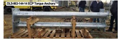
technical soil data and the foundation loading criteria to ECP. The ECP team designed and fabricated a custom Torque Anchor™ Helical Pile foundation that would meet the design criteria, and a pile system that could be installed using an A&N line truck with torque motor. The custom ECP Torque Anchor™ piles were rotated into the soil until reaching stable soil at 12 foot depth.
