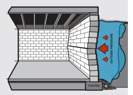
**Bowed Walls** are caused by soil load and under designed foundations. Outside pressure is directed towards the middle of the foundation wall. In order to correct this the wall needs added support so the outside pressure is dispersed throughout the entire wall.
