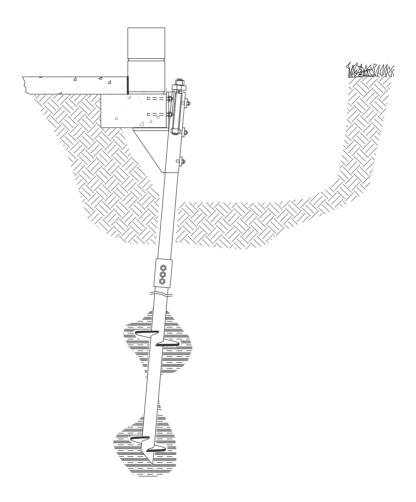
Medium Utility Bracket on Spread footing with block wall
