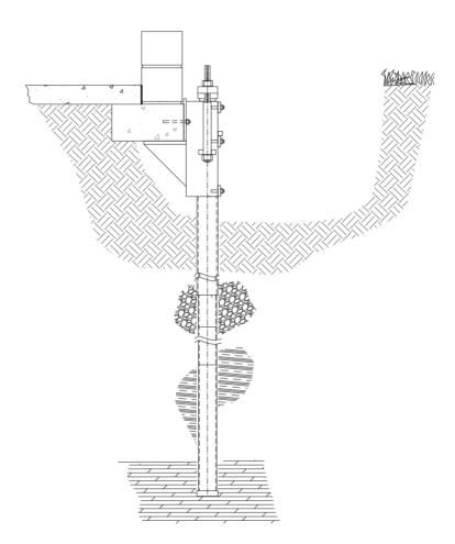
PPB-450EP2 on Spread footing with block wall
