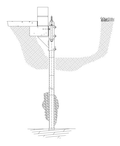
PPB-350 on Spread footing with block wall
