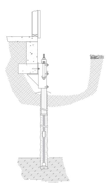
PPB-350MP on Spread footing with concrete wall and raised slab
