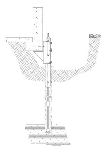
PPB-350MP on Spread footing with concrete wall
