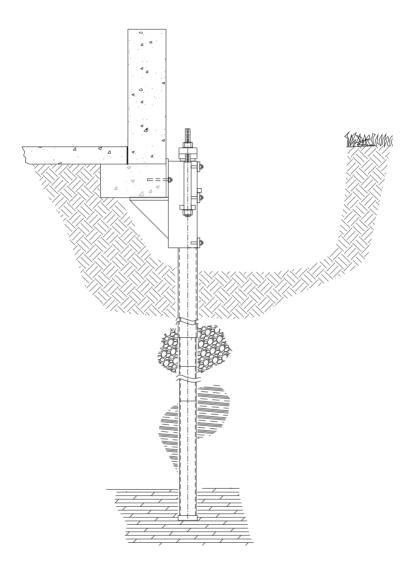
PPB-350EP2 on Spread footing with concrete wall
