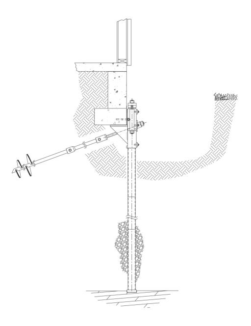
PPB-350-TA on Spread footing with concrete wall and raised slab
