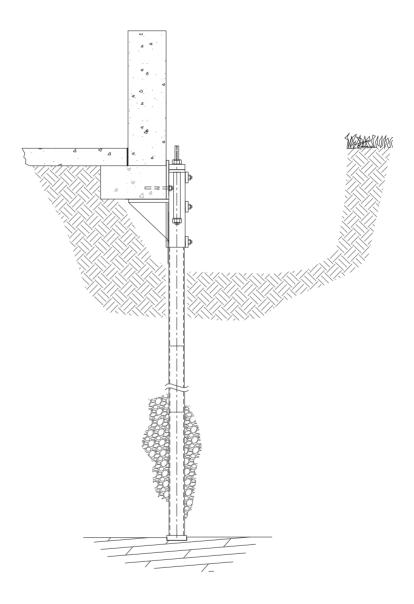
PPB-300 on Spread footing with concrete wall
