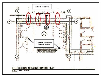
ECP Torque Anchors<sup>™</sup> were used to stabilize an existing 13 foot tall foundation wall during excavation for an addition to the church. The engineer calculated that each Torque Anchor<sup>™</sup> wall placement required to support 30,000 pounds lateral force. A factor of safety of two was specified. Calculations determined that the concrete wall would be able to support a span of eight feet between helical tieback anchors.
