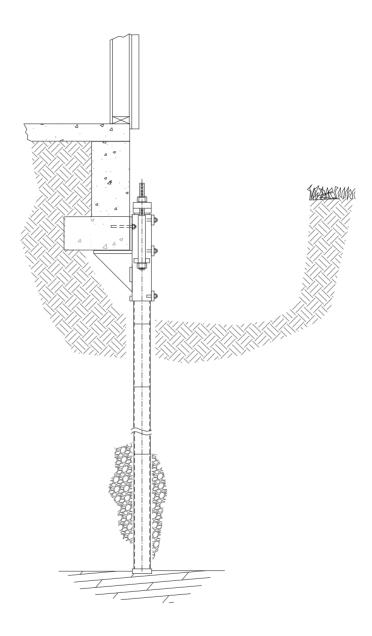
PPB-400 on Spread footing with concrete wall and raised slab
