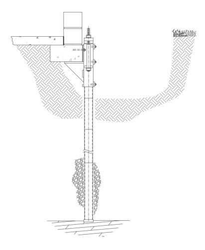
PPB-400 on Spread footing with block wall
