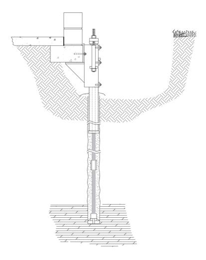
PPB-350MP on Spread footing with block wall
