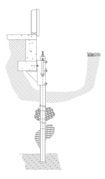
PPB-350EP2 on Spread footing with concrete wall and raised slab
