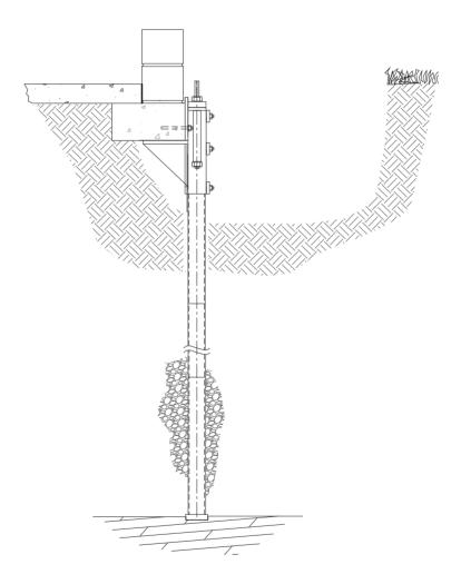
PPB-300 on Spread footing with block wall
