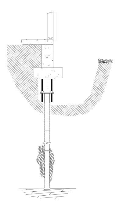
PPB-250 on Spread footing with concrete wall and raised slab
