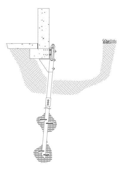
Large Utility Bracket on Spread footing with concrete wall
