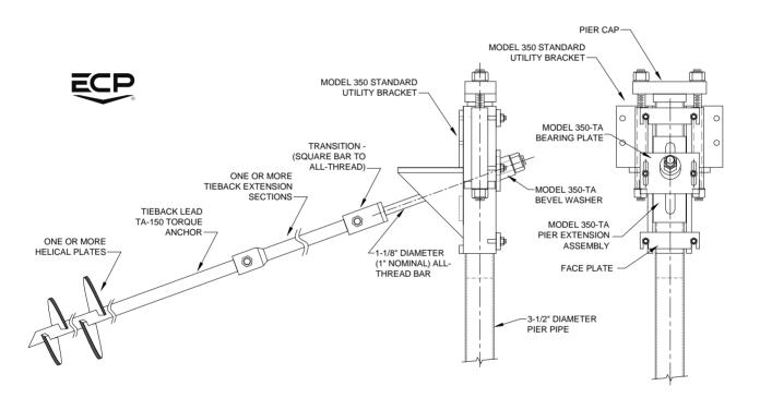
Model 350 ECP Steel Pier<sup>™</sup> System, ECP TA-150 Torque Anchor<sup>™</sup> Tieback and Model 350-TA Tieback Adapter Assembly
