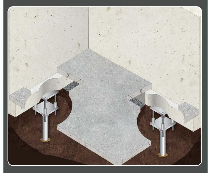
The ECP Steel Push Pier System is a permanent solution for your home's settling foundation. It provides you the very best option to repair your foundation back to level. Steel piers are hydraulically driven through our patented steel bracket to a load bearing stratum, as the entire structure works as the reaction.
